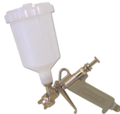
**Model Z3**, internal mixing spray gun, gravity operating with air valve lever. Knurled adjusting screw at the end, adjustable head and round jet. Nickel plated brass body, black anodised aluminium handle.
